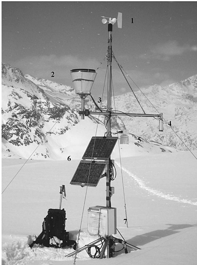
FIGURE 2. AWS1 Forni. The instruments are marked with numbers: (1) wind speed and direction, (2) rain gauge, (3) net radiometer CNR1, (4) sonic ranger, (5) thermo-hygrometer, (6) solar panels, and (7) barometer inside the datalogger box (photo by G. Diolaiuti).
