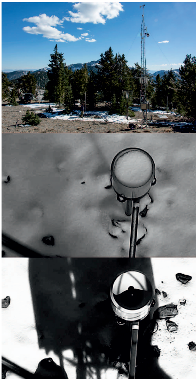
FIGURE 3 Using a webcam as part of an environmental sensor deployment (top) allows the operator to capture images that assist data quality control. In this case, hourly images can show if precipitation is in solid form (middle), which is not usually captured properly by instruments such as a liquid tipping bucket gauge (bottom). (Photos by Scotty Strachan/NevCAN automated systems)
