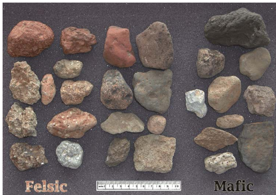
Figure 8. Felsic rocks (left) and mafic rocks (right) are often distinguished by the presence or absence of large crystals, the color of the crystals and the matrix rock, and surface texture. Intermediate varieties (center) are particularly difficult to classify based on such attributes. A precise identification requires chemical analysis.
