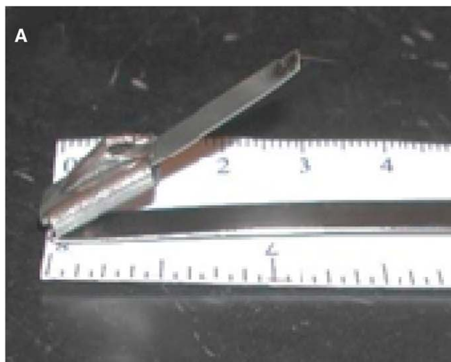
Fig. A2. Attaching the dendrometer band collar. (A) Slip a collar on the short section with the “tab” end of the collar away from the bend. (B) Fold the protruding short end of band under the collar and crimp the folds to secure the collar.
