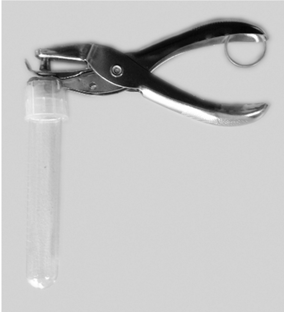
Fig. 3. Modified single-hole punch to collect pooled leaf samples as described in Appendix 1, Note 8.
