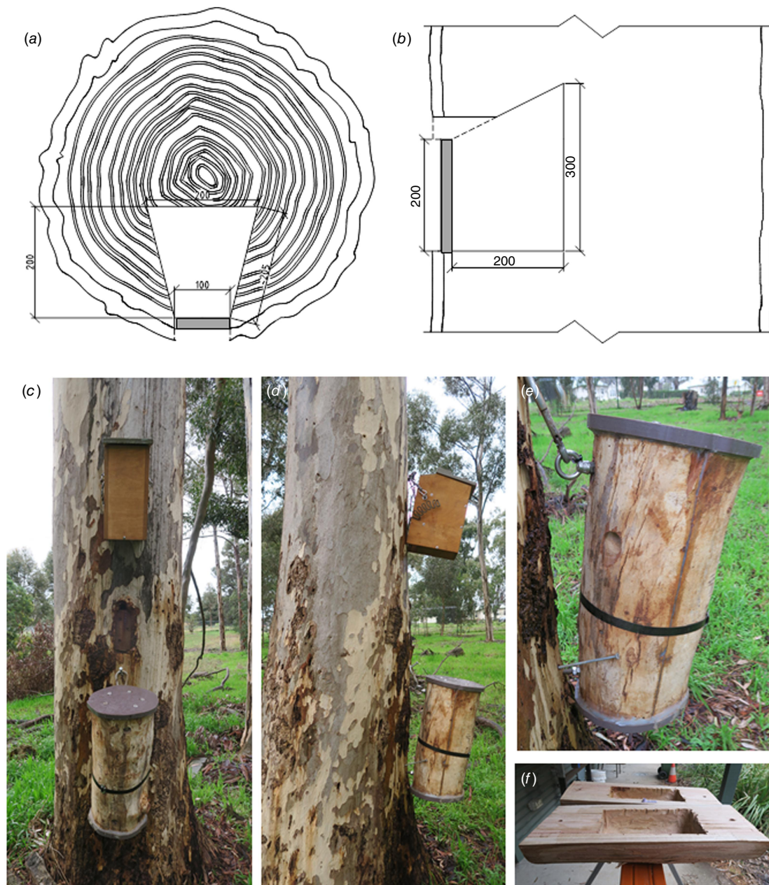
Fig. 2. Diagram of a trapezoid prism-shaped chainsaw hollow cavity showing (a) cross-section and (b) side views of the trunk (cavity dimensions shown are in mm); grey-shaded rectangles represent the pre-made hardwood faceplate (100 × 200 × 30 mm, width × height × depth; adapted from Best et al. 2022). (c, d) An example of a nest box (1.5 cm thick marine plywood; internal cavity dimensions 15 × 35 × 16 cm, width × height × depth; cavity volume = 8400 cm 3 ), log hollow (mean ± s.d. dimensions of the eight logs: length = 60 ± 3 cm; diameter = 31 ± 2 cm; cavity volume = 6343 ± 675 cm 3 ) and chainsaw hollow (mean volume of the eight cavities = 6258 ± 892 cm 3 ) installed on a single tree (sugar gum, E. cladocalyx ); all artificial hollows had a 3.5 cm diameter entrance hole; the nest box and (e) LH entrances faced the trunk. (f) Internal view of a cylindrical cavity carved into a log hollow.
