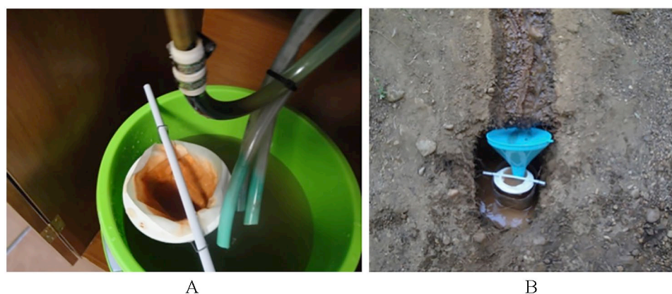
Figure 4. Collection of filters for the soil loss tests in both drainage systems: (A) model and (B) natural terrain.
