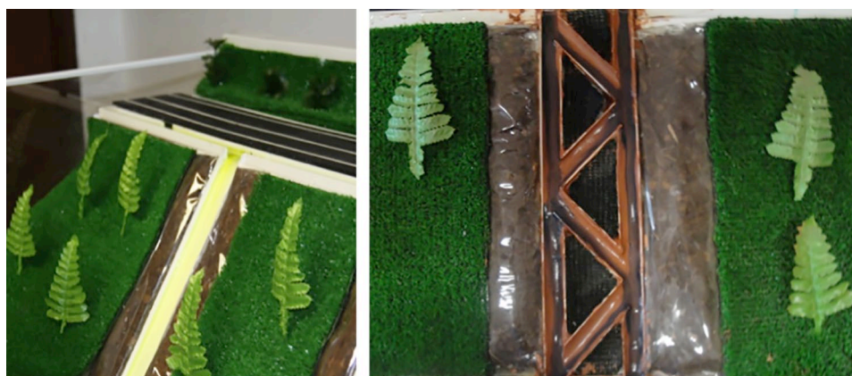
Figure 2. Photographs of the tests performed for the calculation of the average water velocity over the traditional system on polyvinyl chloride (left) and the branched drainage on clay (right).
