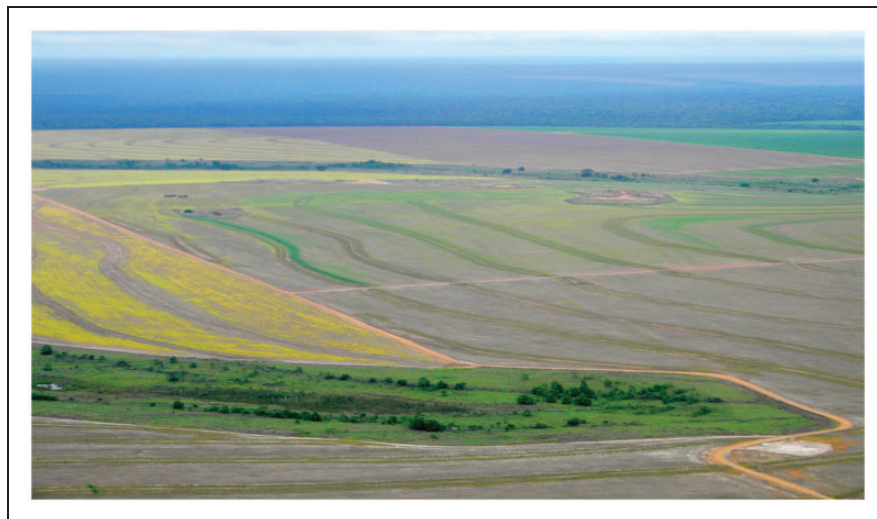
Figure 1. The commercial cropland landscape at Tanguro Ranch in Mato Grosso. Lighter soil strips are locations where contour erosion control berms were removed in 2013 (2 years after installation) to facilitate planting and harvesting. The utility of contour berms was limited because very high rates of soil water infiltration minimized surface runoff. Dark linear features running through cropland are headwater streams and adjacent riparian forests within cropland watersheds. Photo: P. Brando.
