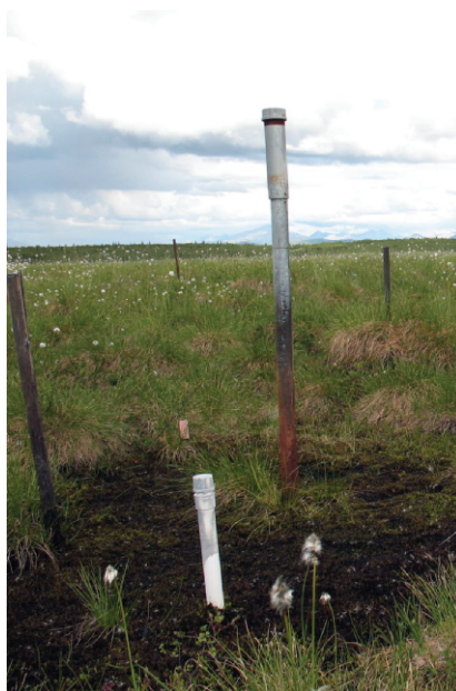
Each year the permafrost temperature at this bore hole gets measured. Photograph: Amy Mayer.
