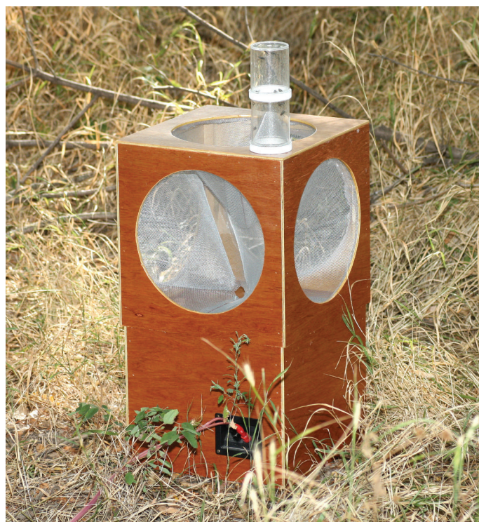
Fig. 1. The complete live trap deployed in the field. Captured flies are visible in the holding jar assembly at the top of the trap box.
