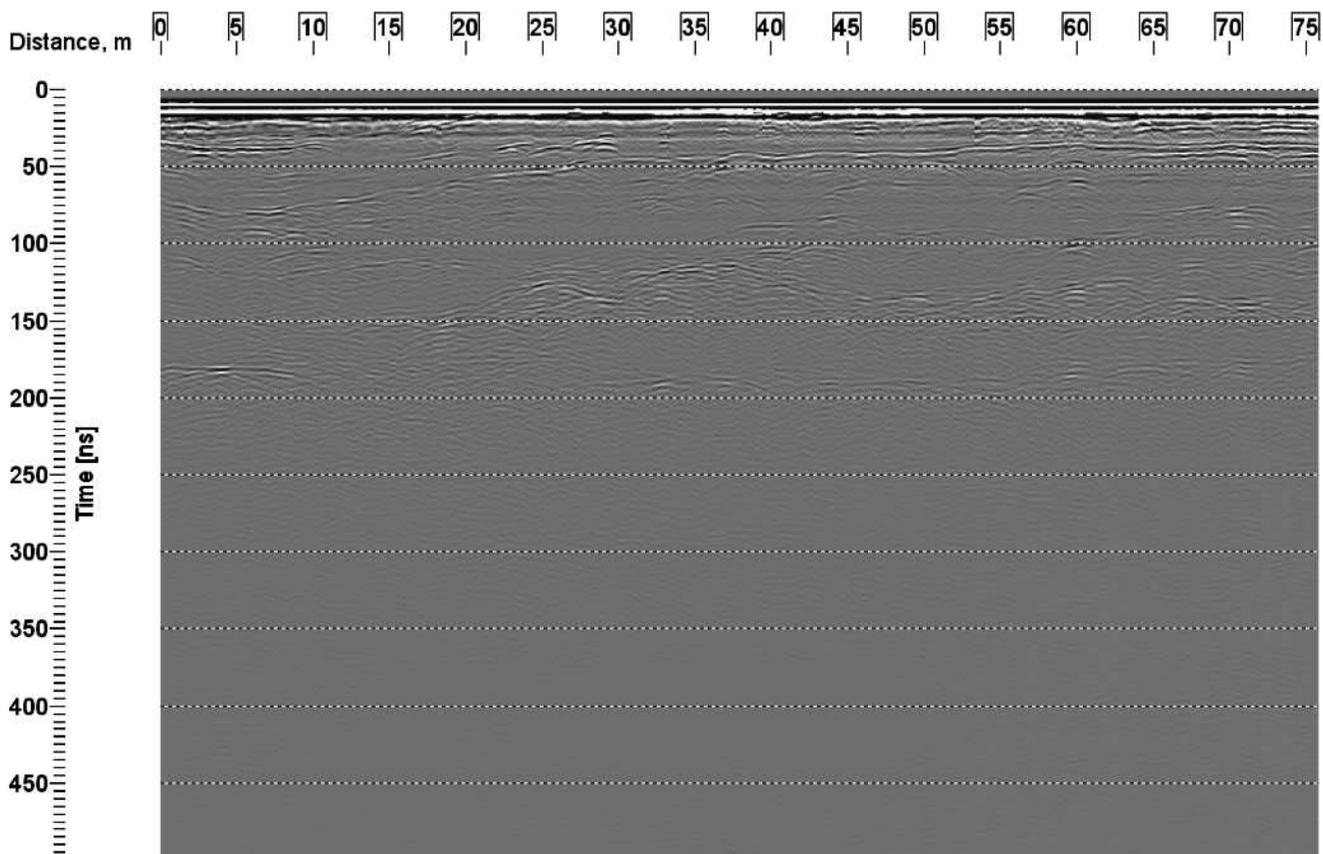
**FIGURE 7.** Raw GPR subsurface profile (transect 1) from 29 October 2007. Strong direct wave reflections are visible at the top of the profile, followed at depth by weaker subsurface reflections. Note the decreasing amplitude of reflections with increased time (depth) as a result of signal spreading and absorption.
