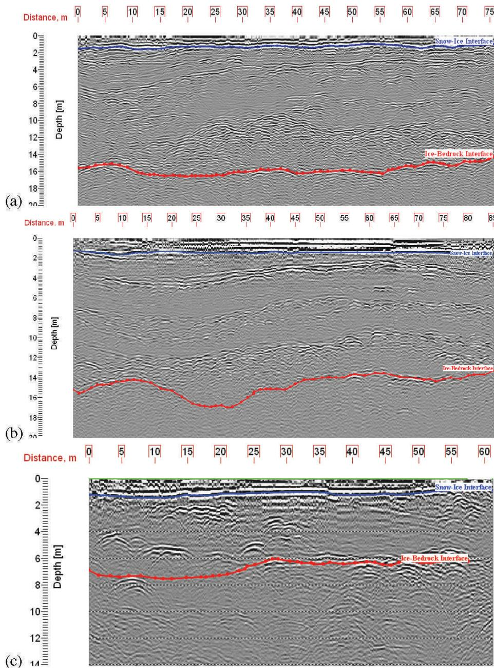
**FIGURE 8.1.** Processed and interpreted contour-parallel sub-surface profiles 1 (a), 2 (b), and 4 (c). The snow-ice interface and basal contact of the glacier are shown. Note the  $\sim 10$  m decrease in depth to the basal contact between profiles 1 and 2 and profile 4. Ice layers and entrained rock debris are visible in all profiles. Vertical exaggerations in (a), (b), and (c) are 1.4, 2.7, and 2.0, respectively.
