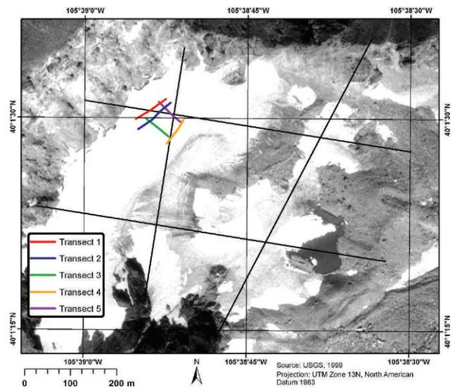
**FIGURE 6.** GPR transect lines projected on the aerial photograph from 13 September 1999. NE–SW trending transects run approximately parallel to topographic contours, NW–SE trending transects run approximately perpendicular. Actual transects intersect at all possible points. Discrepancy in projection is due to handheld GPS point uncertainties.
