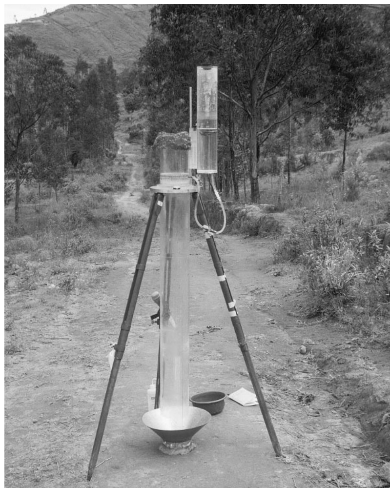
FIGURE 2 Use of a rainfall simulator-infiltrometer on a trail near Quito, Ecuador. (Photo by author)
