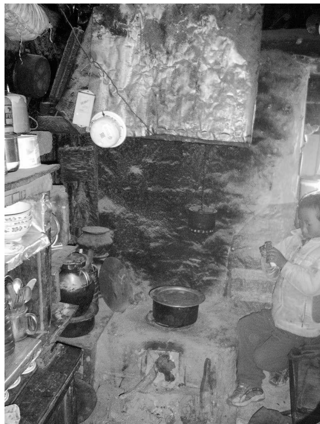
FIGURE 5 A traditional metal stove without a chimney in a residential house in Thame. (Photo by Atindra Sapkota)
