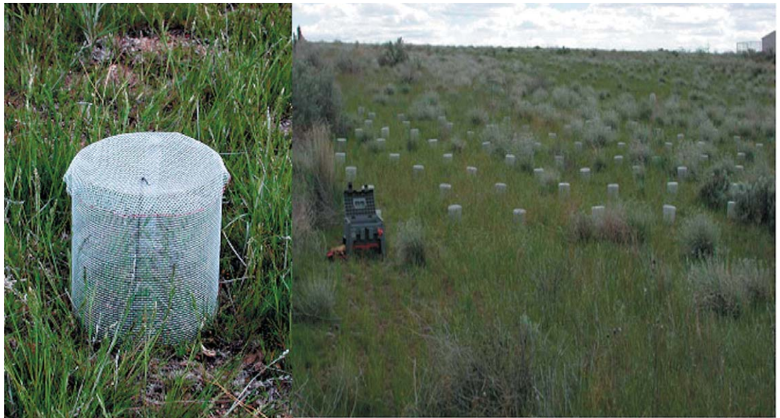
Fig. 1. a) (left) Close up of hardware cloth cage used to contain Mormon crickets exposed to sprayed vegetation or baits; b) (right) Cages set up on Idaho rangeland.
