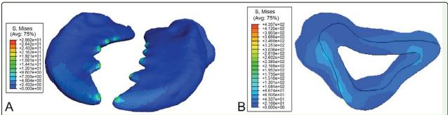
Figure 5. Mandibles of *Priacma serrata* with von Mises stress contours for point load case. (A) Dorsal view. (B) Cross-section of left mandible. High quality figures are available online.
