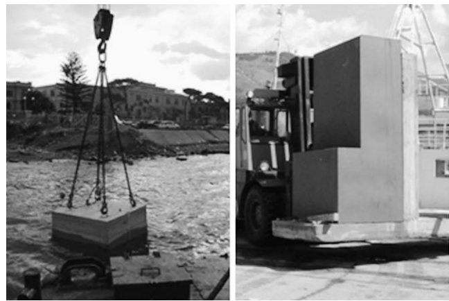
Figure 3. (a) The caisson utilized during the experiment RC-2001. (b) One of the nine modules constituting the absorbing breakwater of the experiment RC-2005.
