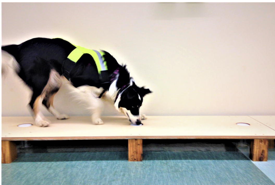
Fig. 2. Platform indicating how containers with breathable lids were placed below the surface and how the platform was used by the detection dog for operant conditioning and during tests.
