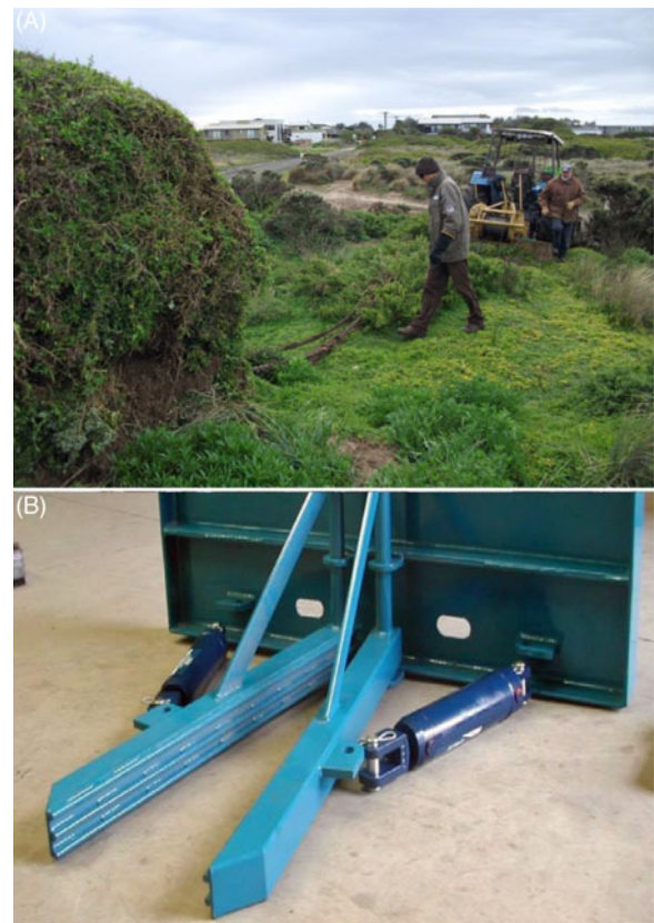
Figure 8. Physical control techniques (A) and machinery (B) for Lycium ferocissimum . (A) Winching out an individual Lycium ferocissimum plant. (B) Lycium ferocissimum puller. (Photo credits: (A) Jon Fallaw; (B) Rob Higgins.)
