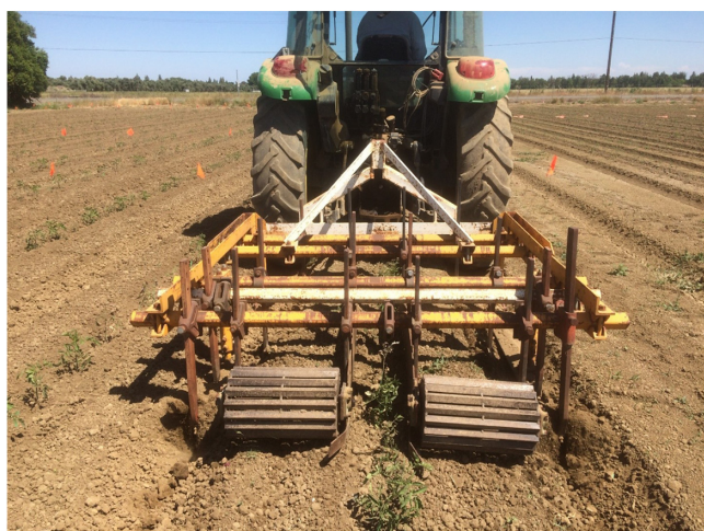
Figure 9. Standard cultivator setup for tomatoes, which left a 15-cm noncultivated band on the crop row.
