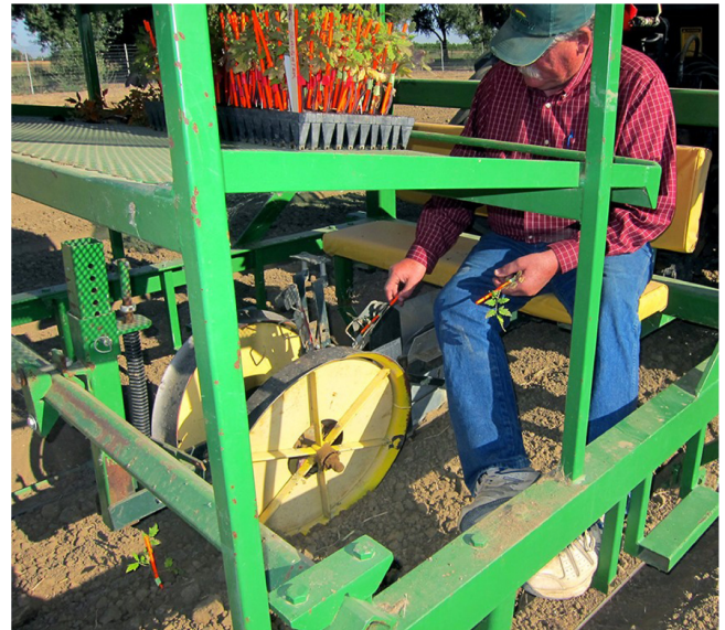
Figure 2. Holland transplanter with butterfly transfer fingers used for transplanting plant labels and tomatoes together.
