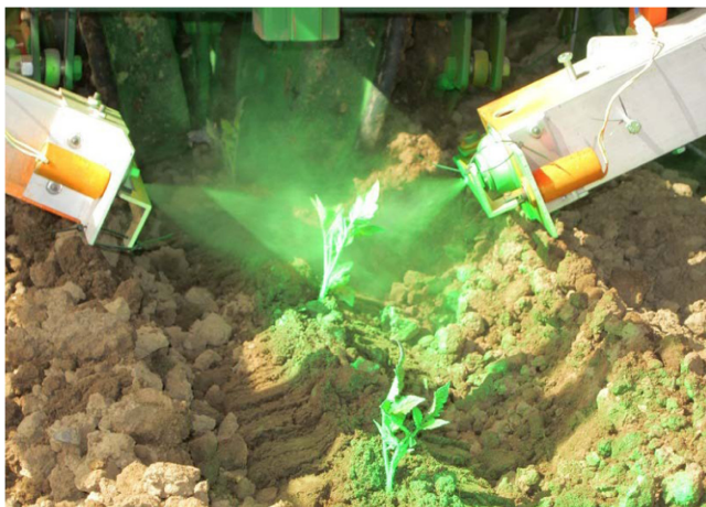
Figure 4. Topical marker sprayed on tomato transplants by applicator mounted on the transplanter during the process of transplanting.
