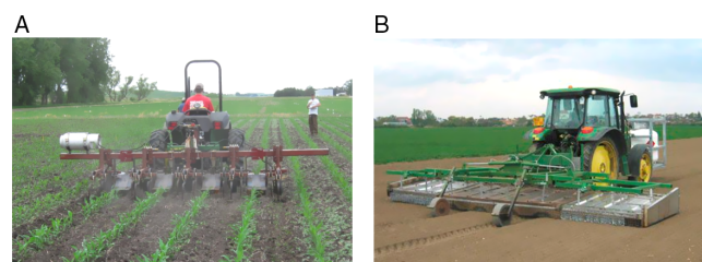
Figure 1. Interrow (left; source Stepanovic [2013]) and broadcast (right; source KULT[2018]) flame weeders in use on early POST maize and PRE vegetable beds, respectively.
