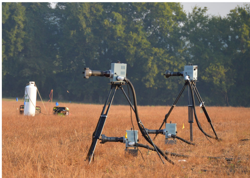
Figure 1. Air samplers shown under field conditions in 2017. Two samplers at 0.3 m height and two samplers at 1.3 m height. Image also shows propane-powered generators used to provide electrical power to operate samplers. Surface treatment shown is dry wheat stubble.
