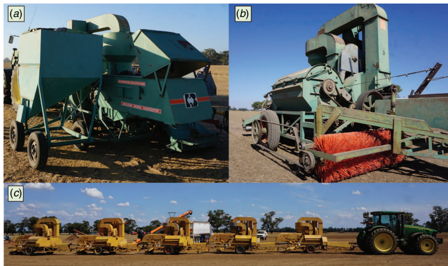
Fig. 7. Examples of Horwood Bagshaw Clover Harvester modifications. (a) An external seed storage bin. (b) Broom ahead of pick-up duct. (c) Tandem drive kit allowing five HBs in a train behind a single tractor.
