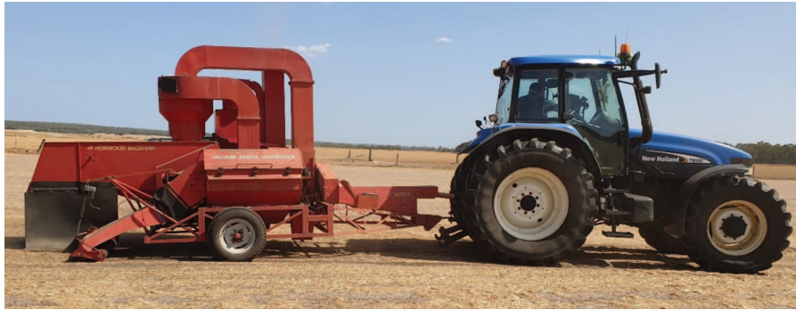
Fig. 1. Horwood Bagshaw Clover Harvester operating in a subterranean clover paddock, 2020.
