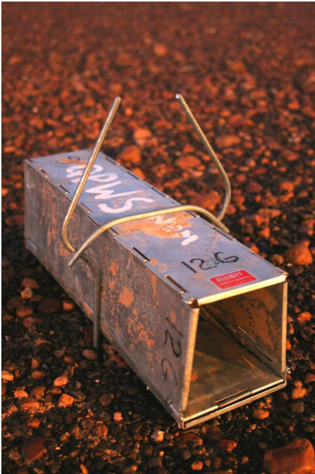
Fig. 2. An Elliott trap with a peg that was developed during the project that could push into the ground and hold the trap in place during wind events.
