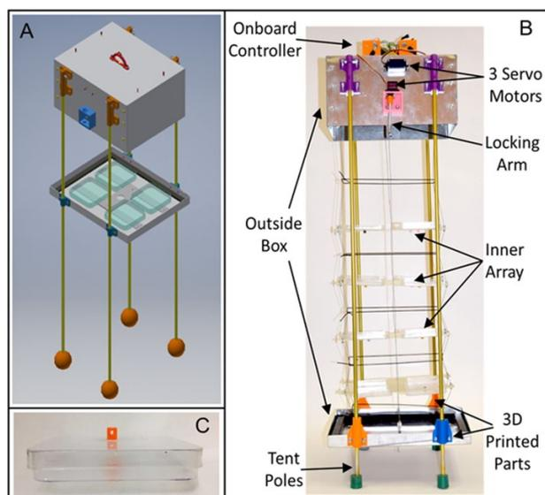
**Figure 2.** Remote Airborne Microbial Passive (RAMP) sampler design. (A) Computer-Aided Drawing (CAD) image of the RAMP sampler box showing array concept. (B) Photo of the RAMP sampler box open showing the features of the sampler. (C) Photo of a collection dish with a 3-dimensional (3D)-printed connector attached.
