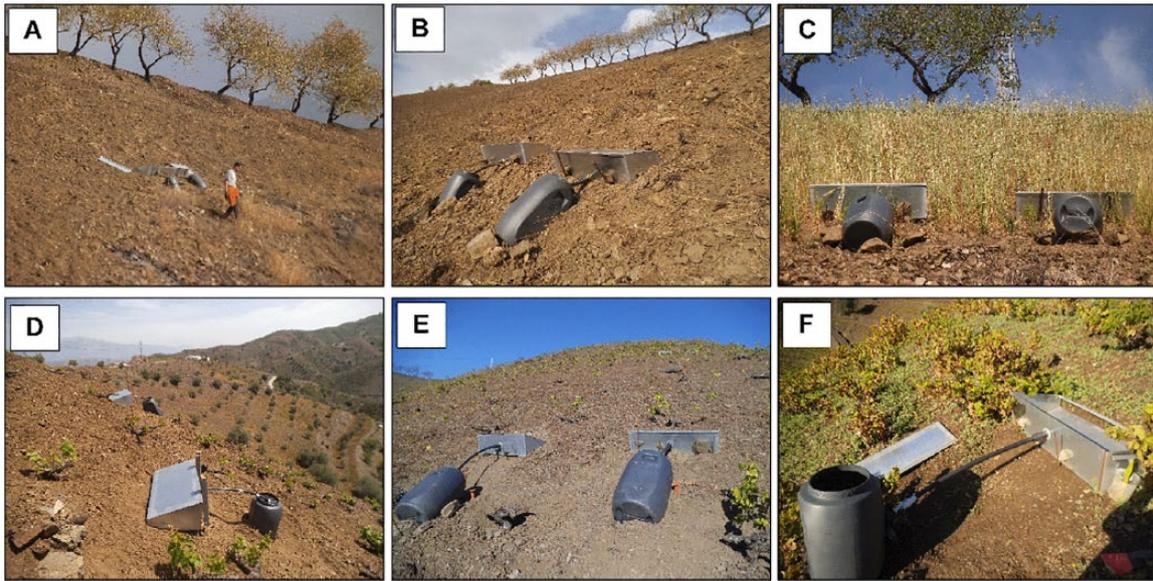
**Figure 2.** General views of the erosion plots: (A) installation of the Gerlach troughs in the abandoned plot; (B) bare soils in the abandoned plot after using herbicides; (C) growing of the barley for the animals; (D) installation of the Gerlach troughs in the cultivated plot; (E) general view of the cultivated plot; and (F) collecting soil erosion results from the cultivated areas after 1 rainfall event.
