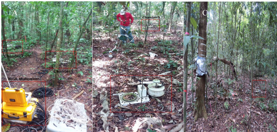
Figure 3. Photographs of the soil flux chambers used in this study: (A) infrared gas analyzer (IRGA) multiplexer device with chambers 1 and 2, (B) chambers 2 and 3, and (C) chamber 4.
