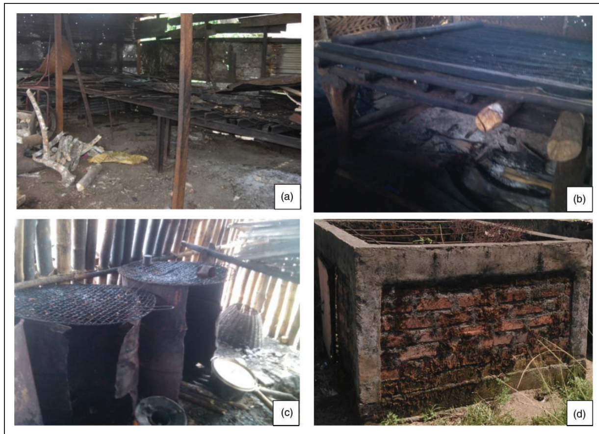
Figure 9. Oven types in study site. (a) Suspended iron banda . (b) Suspended wooden banda . (c) Circular oven. (d) Cinderblock oven.
