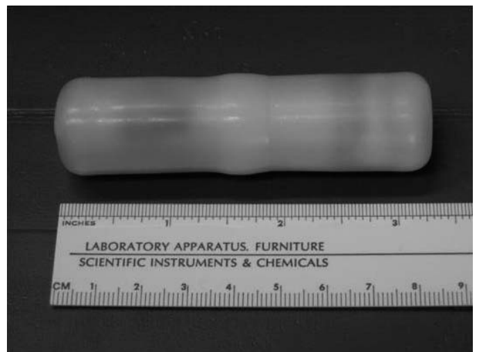
FIG. 2.—Telonics IMP-300-L very-high-frequency transmitter. Transmitters were gas sterilized and subcutaneously implanted into harbor seals.
