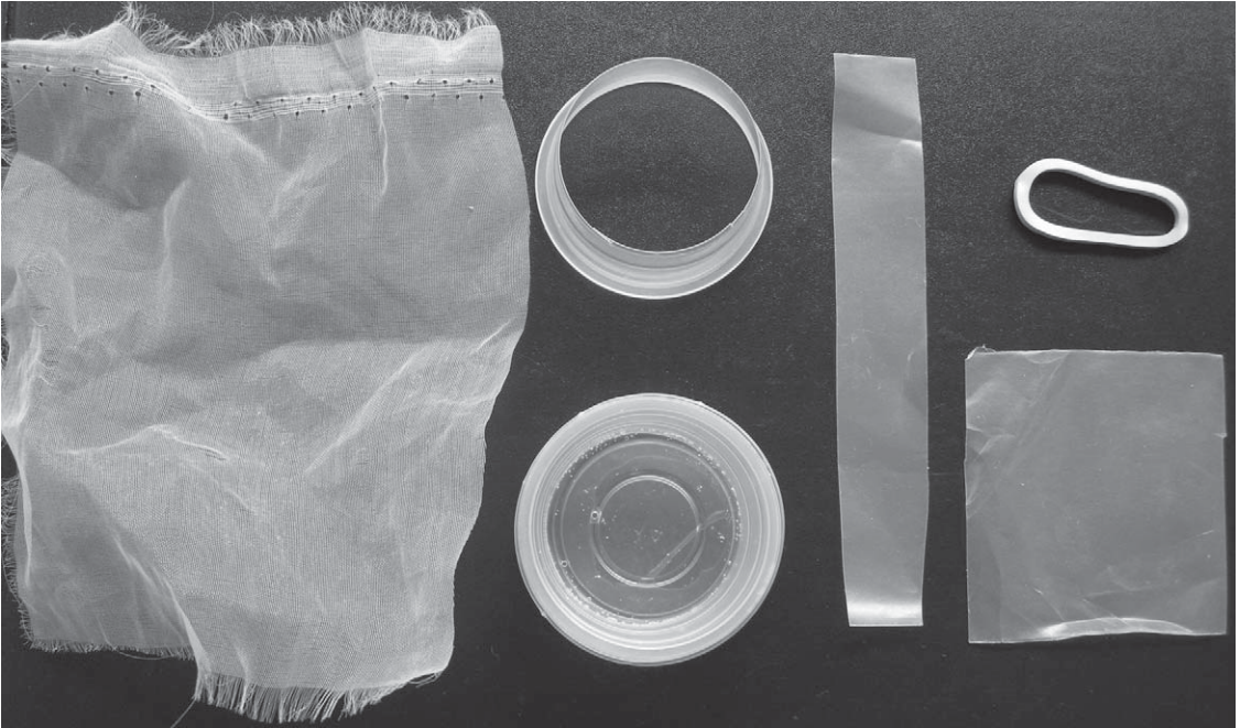
Fig. 1. Material for the assembly of a feeding chamber for Myzus persicae . The feeding chamber was constructed of the following items: 2 plastic tumblers of double-nought number [40 × 20 mm] (1a), one of which is open on both sides (1b), 2 pieces of Parafilm, one of which is larger and more narrow than the other (1c), a rubber band (1d) and a piece of thin fabric (1e).
