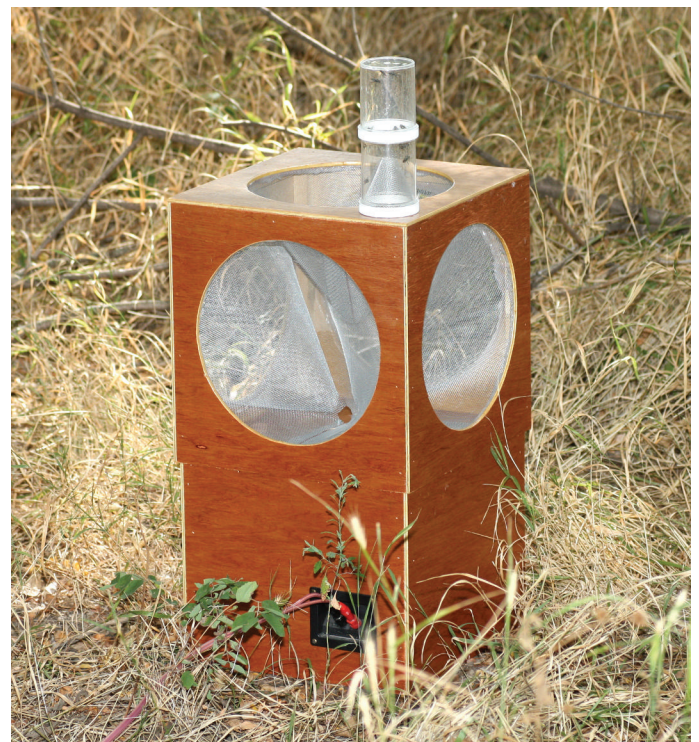
Fig. 1. The complete live trap deployed in the field. Captured flies are visible in the holding jar assembly at the top of the trap box.
