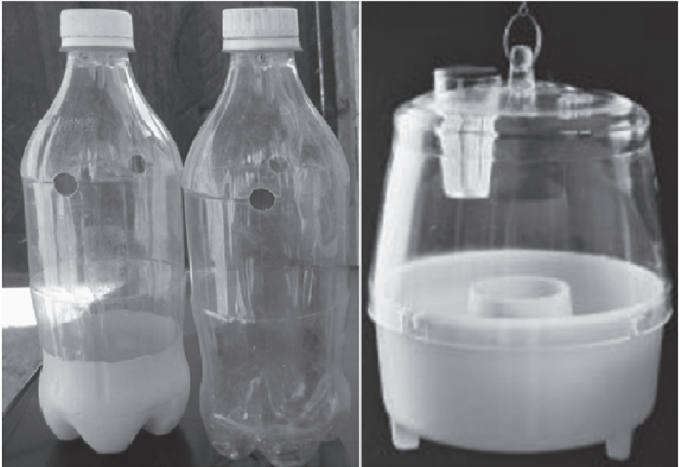
Fig. 1. Trap models developed and used for evaluation of mass trapping efficacy for fruit flies in a mango orchard in Haiti. AT1, yellow-bottomed artisanal trap; AT2, clear artisanal trap; and MP, commercial McPhail trap.
