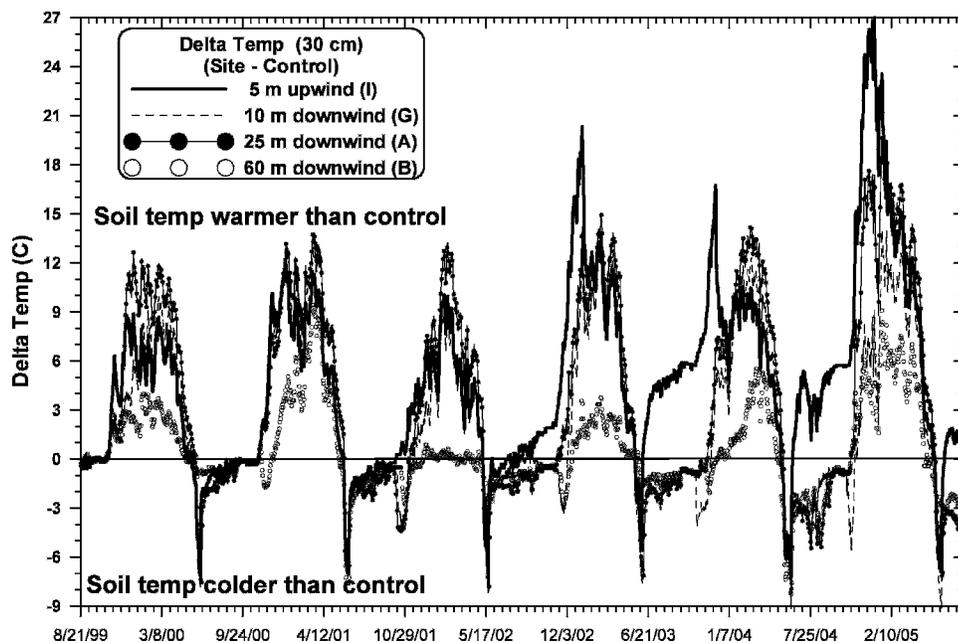
**FIGURE 8.** Difference in soil temperature ( $\Delta T$ ) between Control (average) and four sites for period of record at a depth of 30 cm. Tick marks at 20-d interval. Traces have been slightly smoothed.
