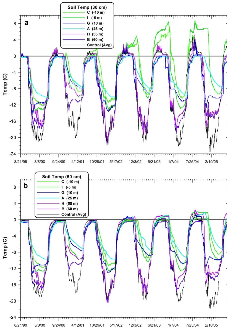
**FIGURE 4.** Soil temperature time series from (a) 30-cm and (b) 50-cm depth for six sites and average Control over period of record (21 August 1999 to 7 August 2005). Tick marks at 20-d interval. Note that some records are discontinuous or are truncated.
