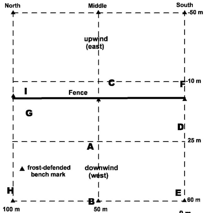
**FIGURE 3.** Study area near southern end of snow fence showing north, middle and south transects. Letters indicate location of thermistor canisters; triangles show position of frost-defended bench marks.
