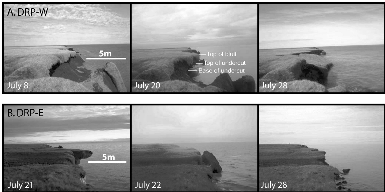
FIGURE 3. Selected images from timelapse sequences at (A) DRP-W and (B) DRP-E cameras. Middle image in DRP-W images shows position of measurement points for quantitative estimates of melt rates shown in Figure 6. DRP-E sequence shows rapid thermal disintegration of ~2-m-wide calved block once it falls into the sea.
