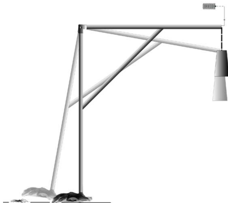
Figure 2. Side view of the lever system used to propel the model frog toward a spider at rest on the water surface (bottom left). At the start of a trial, the horizontal arm is released by a solenoid (top right), the suspended mass accelerates downward, and the model frog accelerates to the left.
