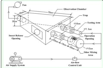
**Figure 1.** A schematic representation of the olfactometer. High quality figures are available online.
