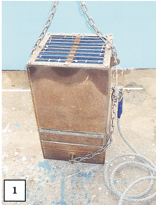
Fig. 1. Photograph of the dredger used in this study. In this photograph, the dredger is upside down. The dredger was suspended in this position temporarily at 5 m above the sea bottom. When the dredger stopped swinging, it was dropped down to the sea bottom in this upside-down position. The dredger stuck in the mud at the bottom. Then, the rope attached to the side of the dredger was pulled by a winch in order to rotate the dredger in the mud. The dredger with specimens was lifted from the mud in the upright position onto the research ship.
