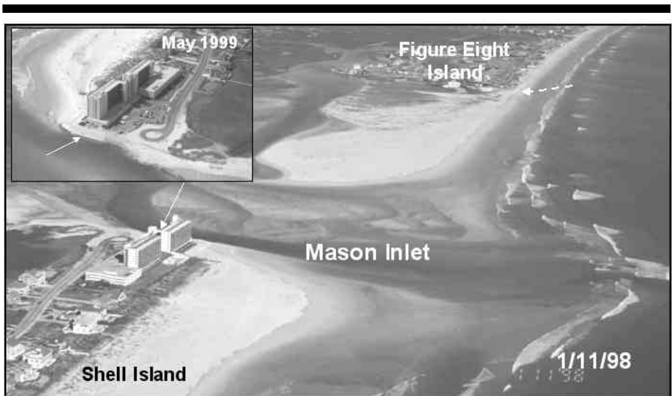
Figure 3. North view (1/11/98) of Mason Inlet and adjacent Figure Eight Island and Wrightsville Beach. Insert (5/99) shows oversized sand bags at base of threatened Shell Island Resort. Note clogged interior channels and position of ebb channel.
