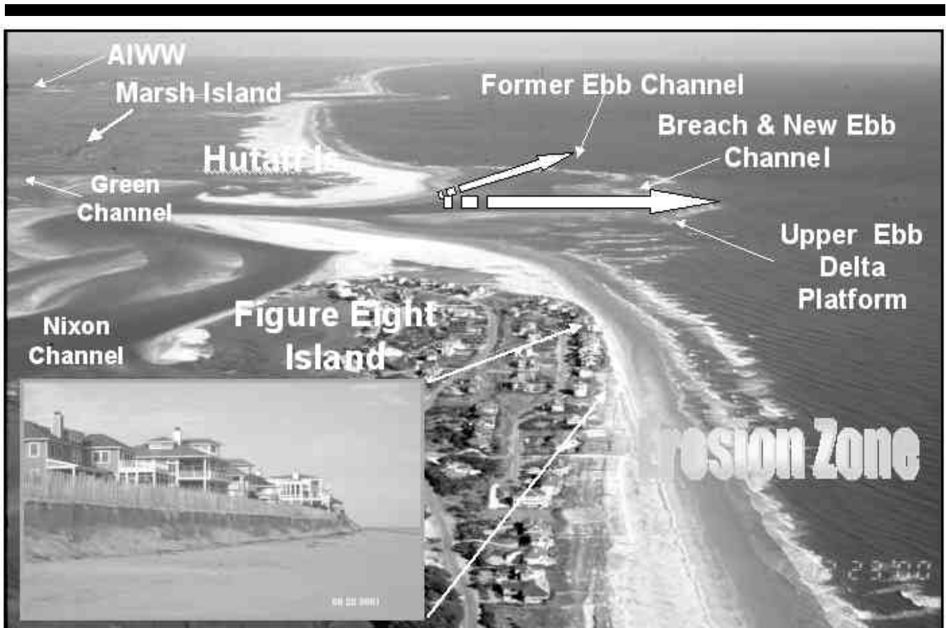
Figure 6. Oblique north view (12/00) of Rich Inlet, Figure Eight Island and Hutaff Island. Rapid erosion of oceanfront stemmed from northeasterly migration and realignment of ebb channel. Ebb delta breaching occurred several months earlier setting the stage for a southerly migration of the channel. Insert shows the current condition (9/01) of the eroding oceanfront.
