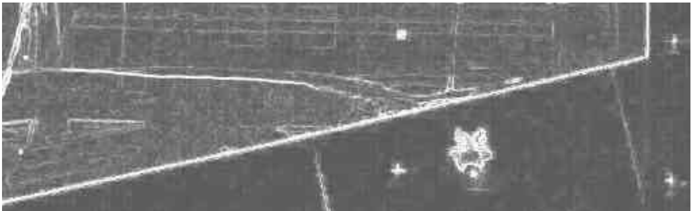
Figure 14. Example non-directional edge detection (Sobel). Control markers can be identified as can the main water surface edge. Note the lack of definition at the turbulent edge and the duplicate edge from the perspective effect, although it is still possible to make out the edge by eye along most of the swash length.
