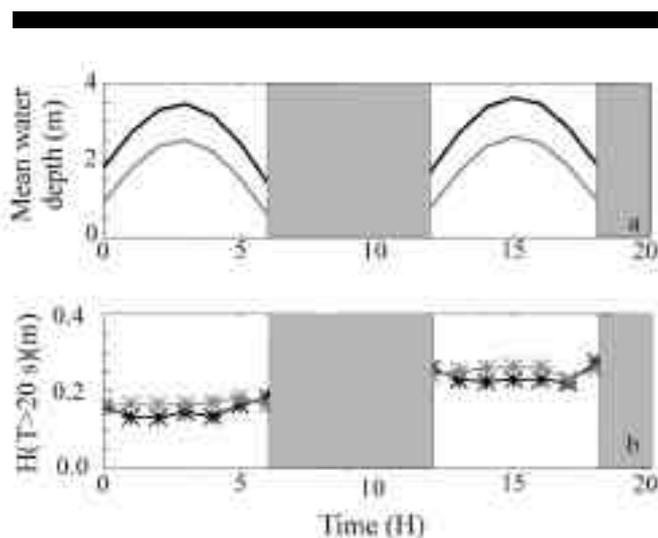
Figure 3. (a) Mean water depth, computed over one hour, versus time (in black: S1 and in grey: S2). (b) Low frequency ( $f < 0.05$  Hz) significant wave heights (computed from the integration of the energy density spectrum in the low frequency band) versus time. The grey rectangle corresponds to the time when the stations were not fully immersed.
