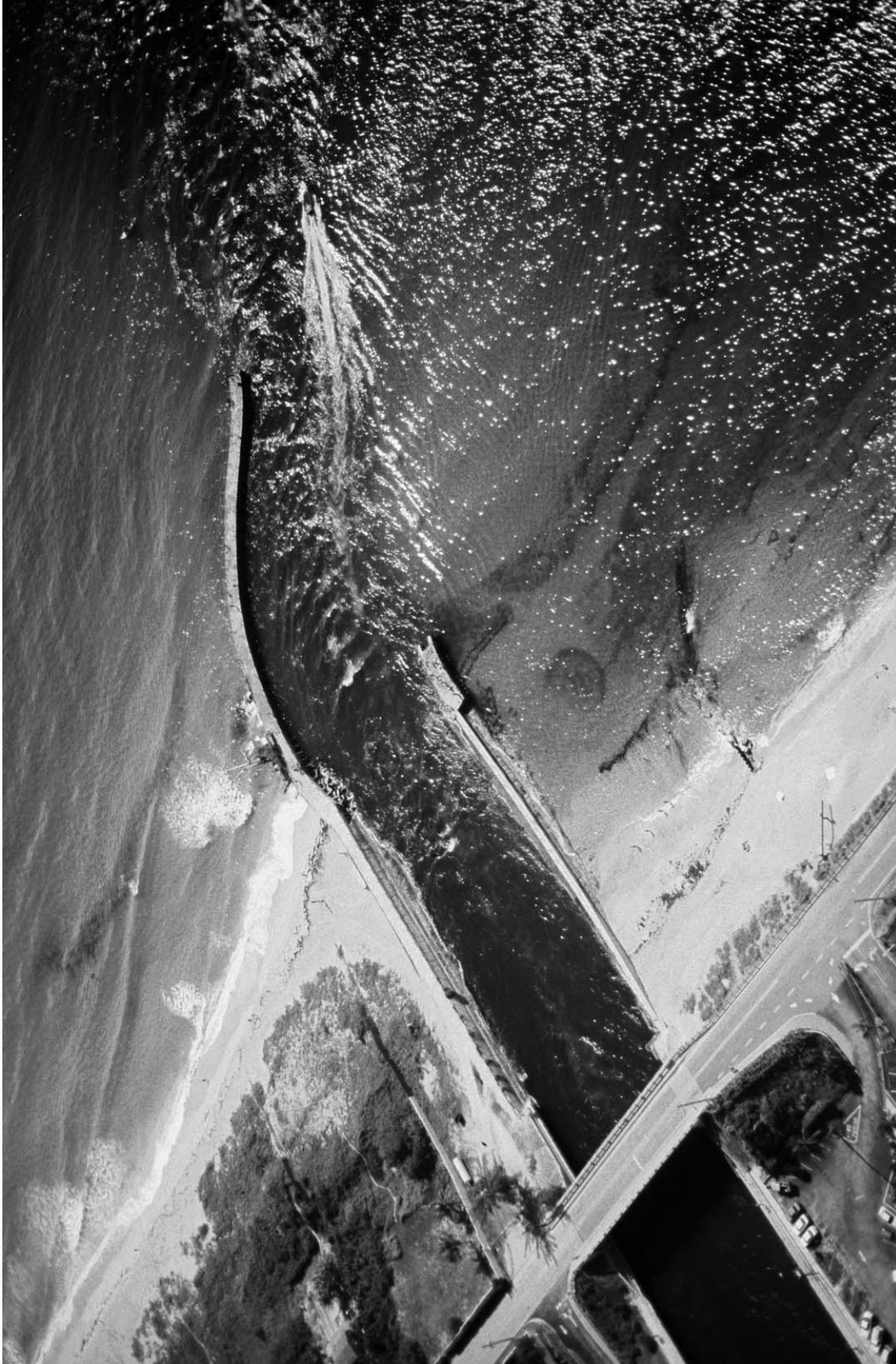
South Lake Worth (Boynton) Inlet on the Southeast Florida Atlantic Coast. This close-up shot shows dark colored tannic acid-rich water flowing out of the Lake Worth lagoon into the Atlantic Ocean. The sand bypassing plant on the shoreward part of the curved north (updrift) jetty pumps sand that accumulates in a fillet as it is impounded by the jetty, which is a littoral drift blocker. Sand is pumped through a pipeline along the north seawall, under the bridge, and then ejected on the eroding downdrift beach. The outlet pipe is visible on the road across from the parking lot (lower left hand corner). (Photograph by Charlie Finkl, Department of Geosciences, Florida Atlantic University, Boca Raton, FL 33431, USA).
