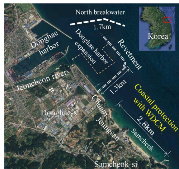
Figure 2. Schematic sketch of Donghae harbor three phase expansion project. Coastal protection with WDCM is planned to Chuam, Jeungsan, and Samcheok beaches located in the south of the harbor.
