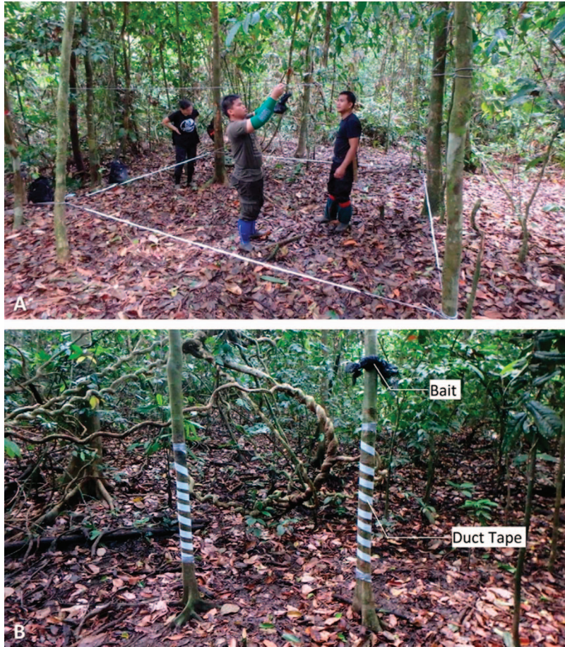
Fig. 2. (a) A hair trap consisting of a duct-taped wire enclosure with bait hung at >1.5 m height to encourage sun bears ( Helarctos malayanus ) to enter the enclosure and make contact with the duct tape; (b) a hair trap consisting of inversed duct tape on a 1.5–1.7-m section of tree where shrimp paste was spread on the tree before wrapping with duct tape. This design encouraged sun bears to stand up on their hind legs to reach the bait, or rub their backs on the tree, exposing their chest mark to the remote camera and depositing hair on the duct tape.
