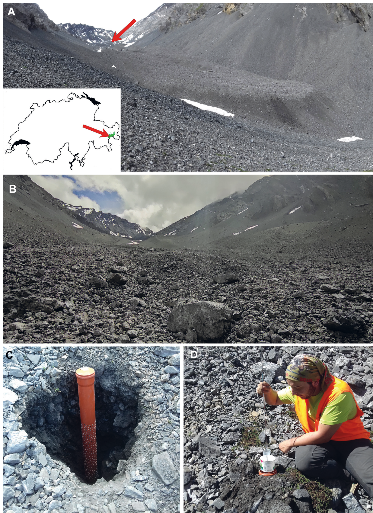
Fig. 1. (A) Location of the sampling site on the rock glacier in Val Sassa in the Swiss National Park. (B) Surface of the rock glacier at the sampling site. (C) Subterranean Sampling Device (SSD) just before burying it. (D) Installation of the pitfall trap in the tube once it was buried.
