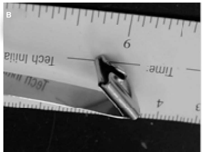
Fig. A2. Attaching the dendrometer band collar. (A) Slip a collar on the short section with the “tab” end of the collar away from the bend. (B) Fold the protruding short end of band under the collar and crimp the folds to secure the collar.
