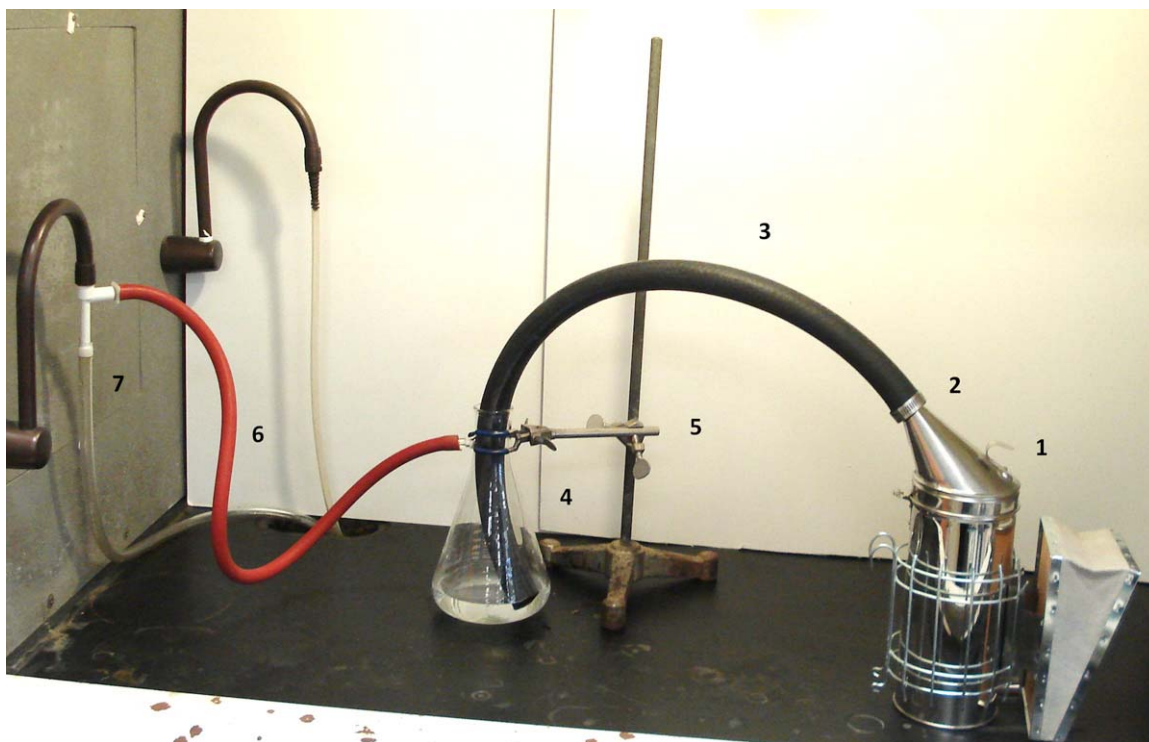
Fig. 1. Smoke solution system. The completed burning system including: (1) bee smoker with bellows, (2) hose clamp, (3) heater hose, (4) side-arm flask, (5) ring stand with clamp, (6) vacuum tubing, and (7) water aspirator. The working system was constructed and used in a fume hood.
