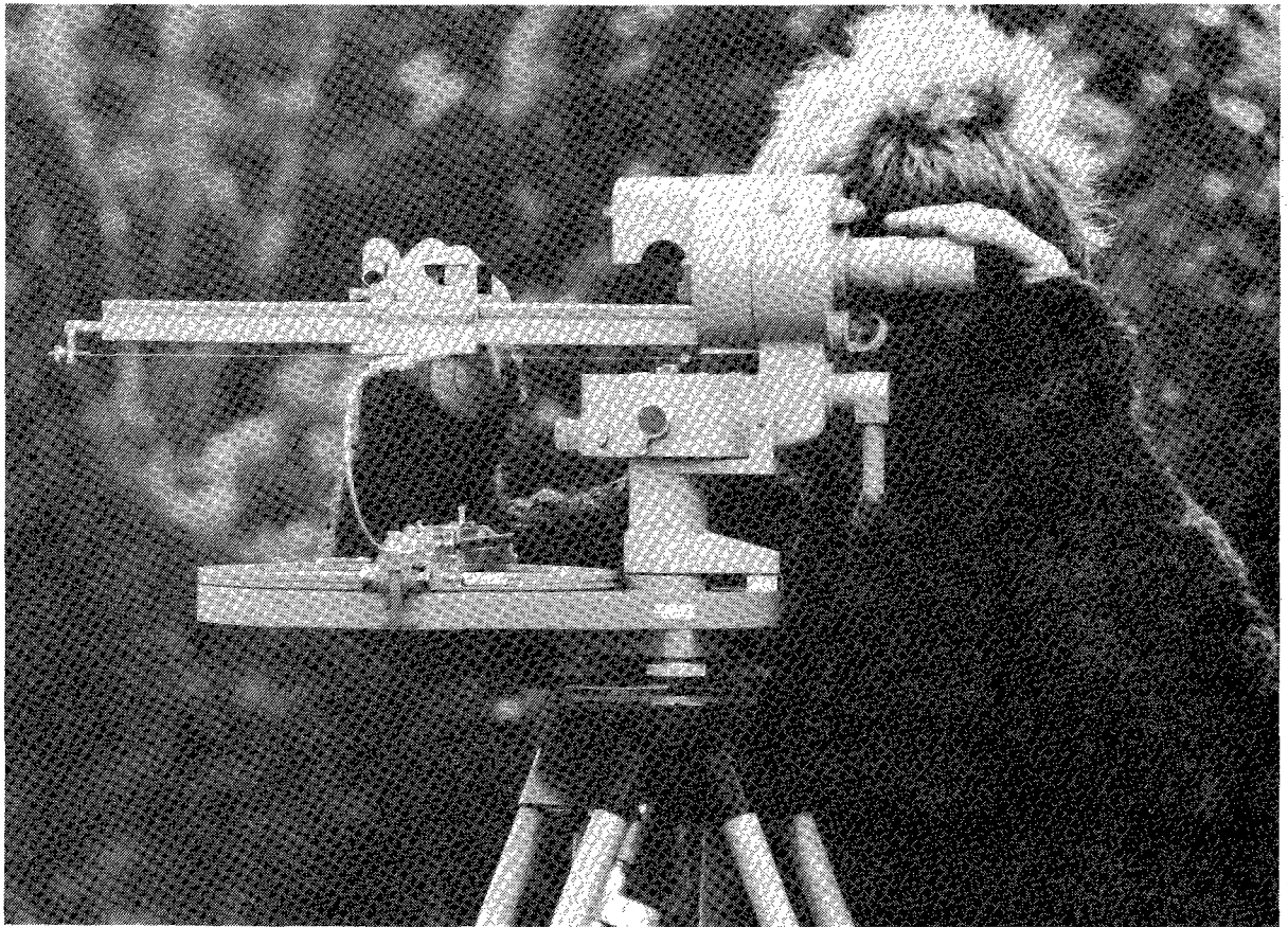
Fig. 25. Optical rangefinder in use for tracking a foraging Starling: the observer brings two images in line by adjusting the movable prism on the side-arm, and the position so obtained is plotted automatically on the circular chart immediately below the arm (sample record in Fig. 27).
