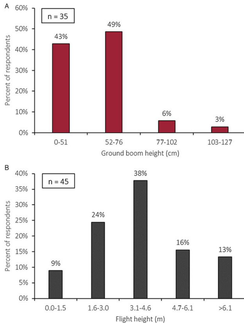
**Figure 4.** Ground spray equipment boom height (A) and agricultural aircraft flight height (B) used for Arkansas agronomic crop herbicide applications as measured by percentage of survey respondents. Percentages may not total 100% due to rounding. The number of total observations is noted in boxes at top left.
