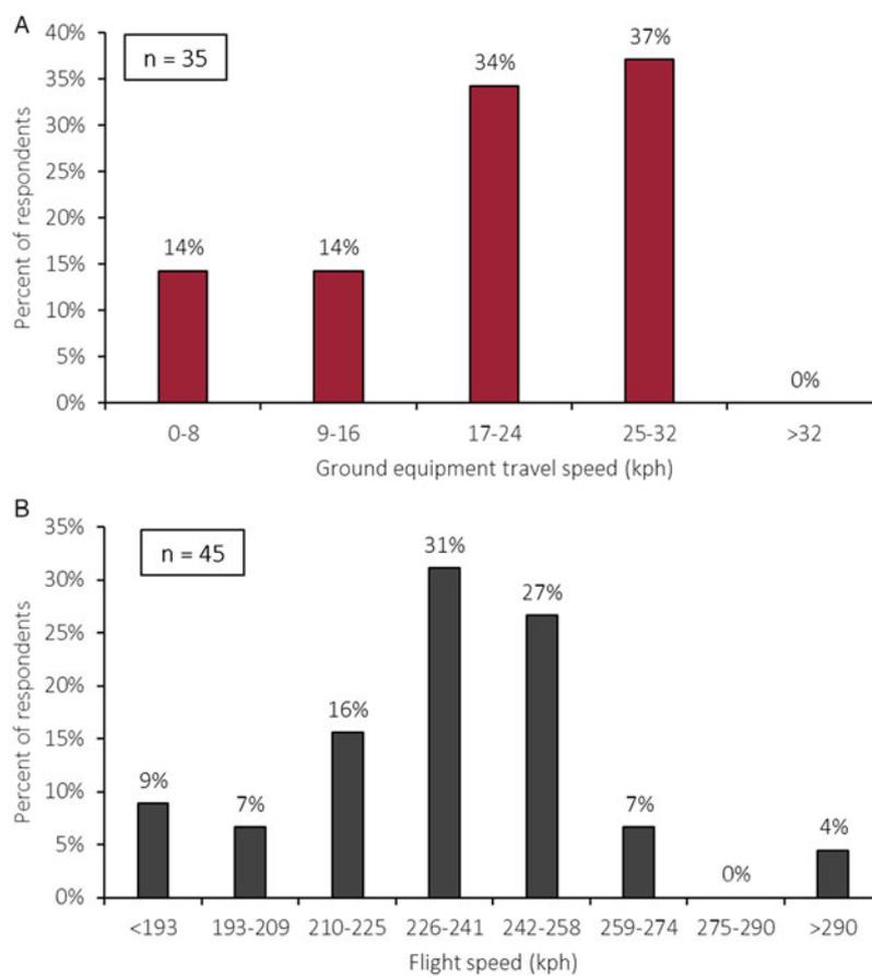
**Figure 5.** Ground spray equipment travel speed (A) and agricultural aircraft flight speed (B) used for Arkansas agronomic crop herbicide applications as measured by percentage of survey respondents. Percentages may not total 100% due to rounding. The number of total observations is noted in boxes at top left.
