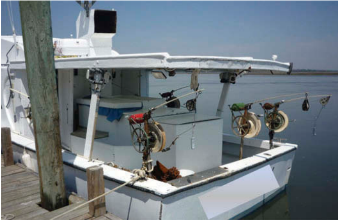
FIGURE 2. Bandit reels attached to the stern deck of a typical commercial snapper–grouper fishing vessel.
