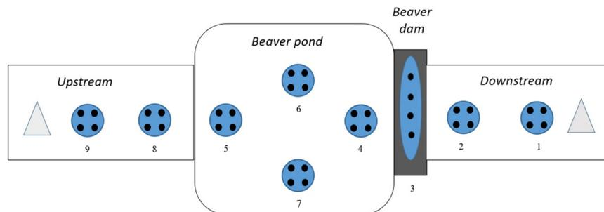
Figure 2. Design of water ( $\triangle$ ) sampling and sediment composite ( $\bullet\bullet\bullet\bullet$ ) sampling in impounded water body. Sampling locations: 1–2 – downstream, 3 – beaver dam, 4–5 – mid-pond, 6–7 – pond periphery, 8–9 upstream.
