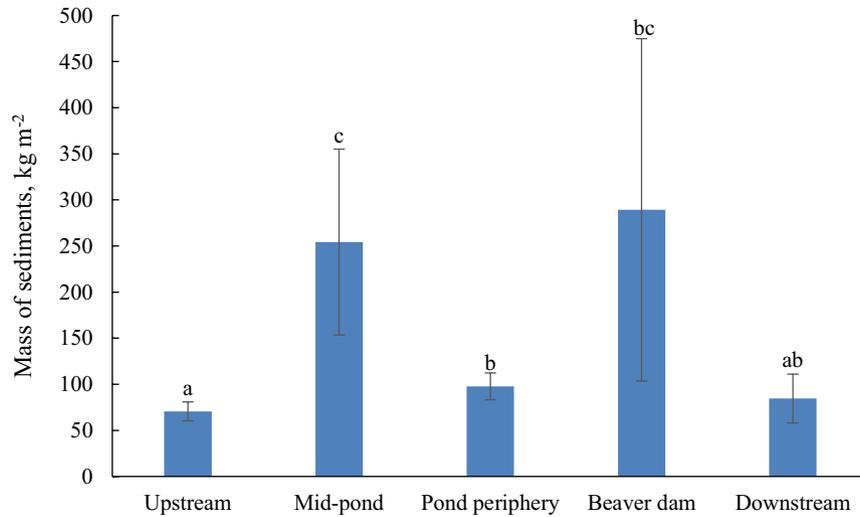
Figure 4. Mean mass of bottom sediments in studied beaver sites in summer (2016–2018). The results are expressed as the mean  $\pm$  SE (total number of samples  $n=81$ , in sampling site: 18 samples were taken upstream; 18 – in the mid-pond; 18 – in periphery of beaver pond; 9 – beaver dam; 18 – downstream). Different lower-case letters indicate significant differences at  $p < 0.05$ .
