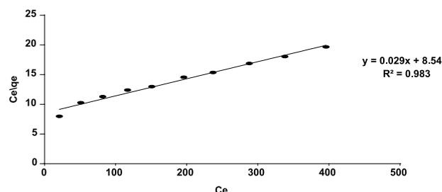
Figure 11. Langmuir isotherm of ascorbic acid removal.
