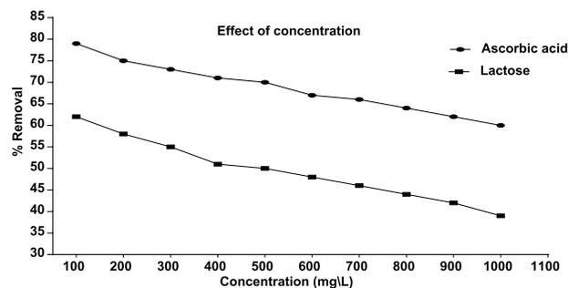
Figure 9. Effect of initial concentration on ascorbic acid and lactose removal.
