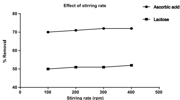
Figure 8. Effect of stirring rate on ascorbic acid and lactose removal.
