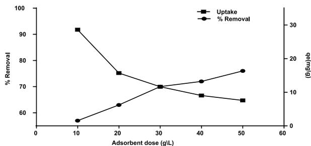
Figure 6. Optimum effective dose for ascorbic acid removal.
